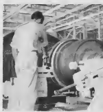
One of the most important jobs being done in the Machine shop when this picture was taken was repair work on a big Powerhouse turbine. Oscar Pieteroz operates the lathe.
